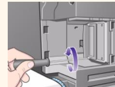
5. When you have inserted the card, screw it into place, using its two screws (at the top and bottom of the card). Again, this can be done with a screwdriver or manually.
