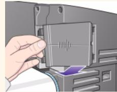
4. To insert a LAN card (or an Accessory card), remove the metal cover from the appropriate slot by unscrewing its two screws. You can use a screwdriver or do it manually.
