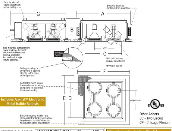
ORDERING EXAMPLE: LV340MHSQ WH 70 120 = Four Light Square Trimless Recessed PAR30MH - White Interior - 70 watt lamps - 120 Volt
