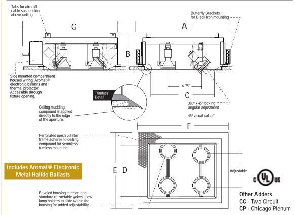
ORDERING EXAMPLE: LV240MHSQ WH 120 = Four Light Square Trimless Recessed PAR20MH - White Interior - 39 watt lamps - 120 Volt
