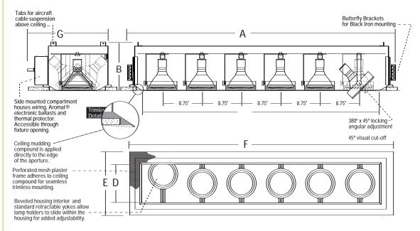
Includes Aromat® Electronic Metal Halide Ballasts
