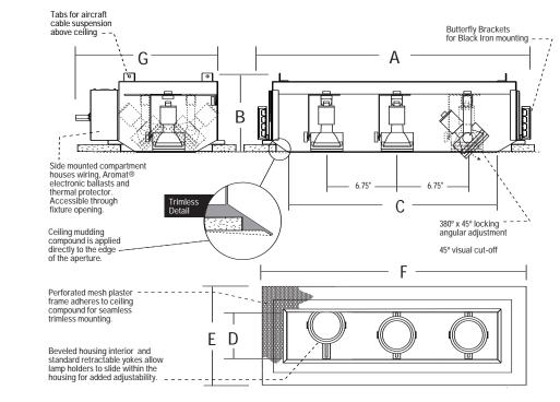
**Includes Aromat® Electronic** Metal Halide Ballasts
