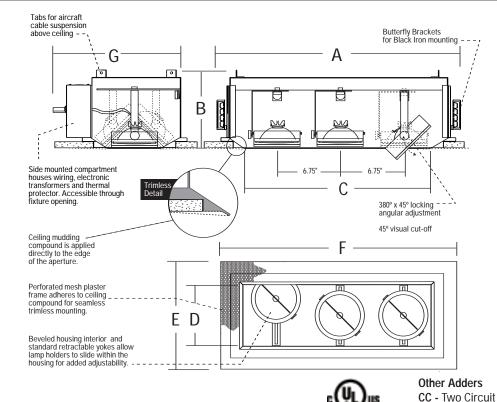
LV1100 WH 50 120 ORDERING EXAMPLE: = Three Light Trimless Recessed AR111 - White Interior - 50 watt lamps -
