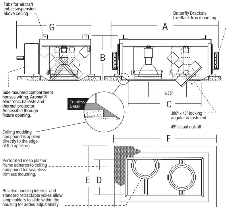
Includes Aromat® Electronic Metal Halide Ballasts
