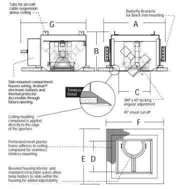
**Includes Aromat® Electronic Metal Halide Ballasts**
