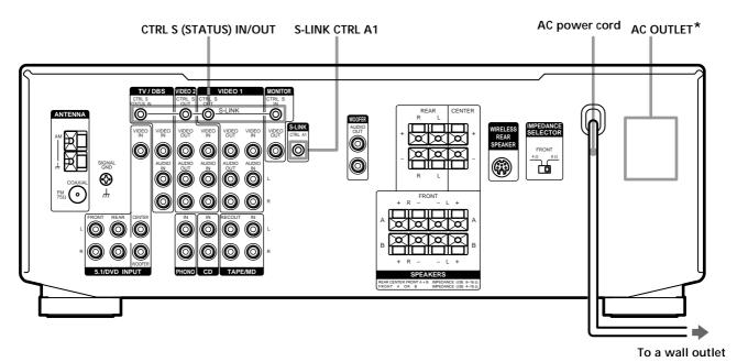
\* The configuration, shape, and number of AC outlets on the rear panel varies according to the model and country to which the receiver is shipped.
