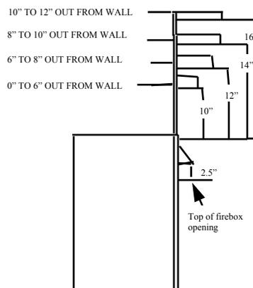
Mantel minimum clearances for a listed Zero Clearance Firebox or a Masonry Fireplace.
