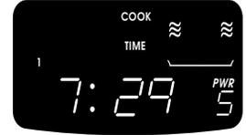
(display counts down cooking time in each cycle, starting with first cycle)
