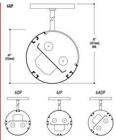
**Construction**: Extruded aluminum housing. Nominal 3', 4', 6' or 8' illuminated sections.
