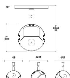
**Construction**: Extruded aluminum housing. Nominal 3', 4', 6' or 8' illuminated sections.
