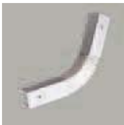
LV215 Flexible Joiner To connect two sections at an angle up to 90° or for connecting wall- and ceiling-mounted sections. Allows for continuation of wireway. May also be used as a feed point. Finish: White (P), Black (MB)
