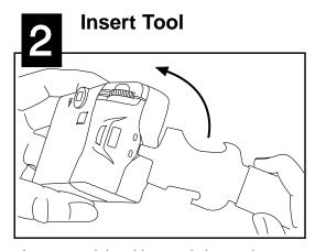
Insert special tool into end slot as shown.
