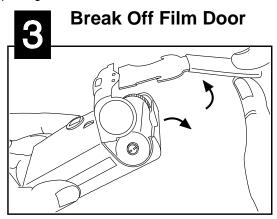
Use tool to break off the film door and remove film.
