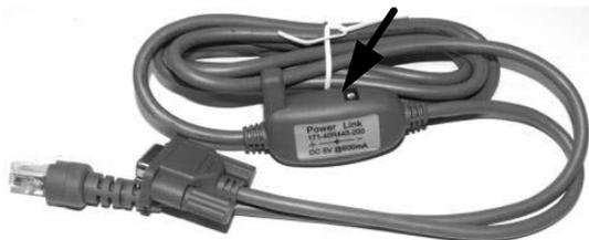
**Fig. 5** RS232 Power Connection
