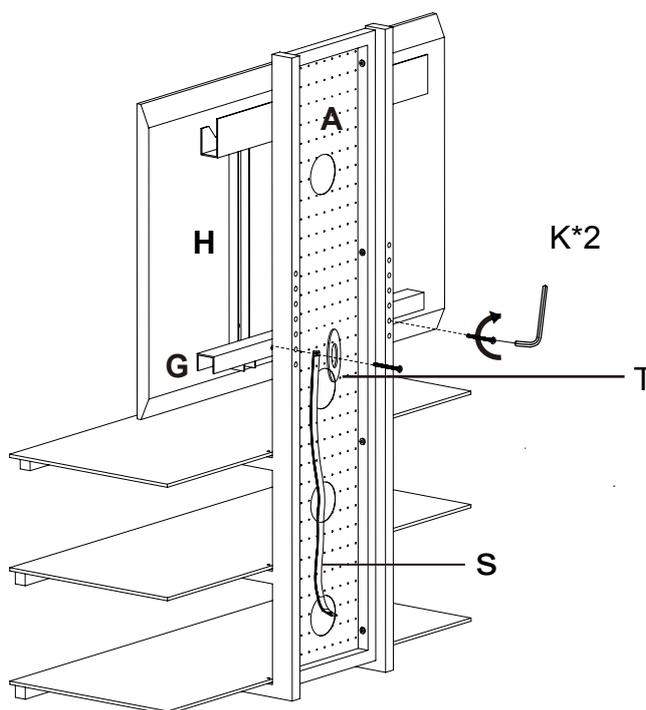
9-Attach holder (G) to bracket (H), fix holder (G) and wall strap(S) to panel (A) with washer(T) and screws (K).
