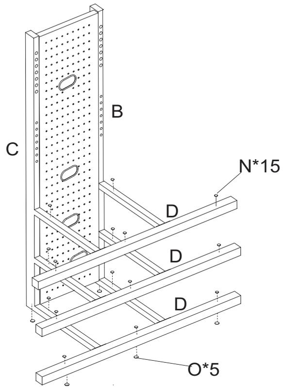
3-Place pads (N) on the beams (D) and frames (B & C). Apply pads (O) at the bottom of the unit.
