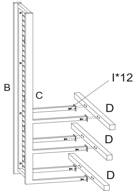
2-Fasten beams (D) to the frames (B & C) with screws (I).
