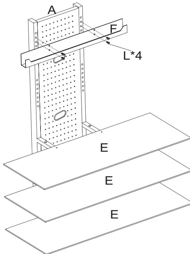
4-Attach holder (F) to panel (A) with screws (L). Place glass (E) on the pads.
