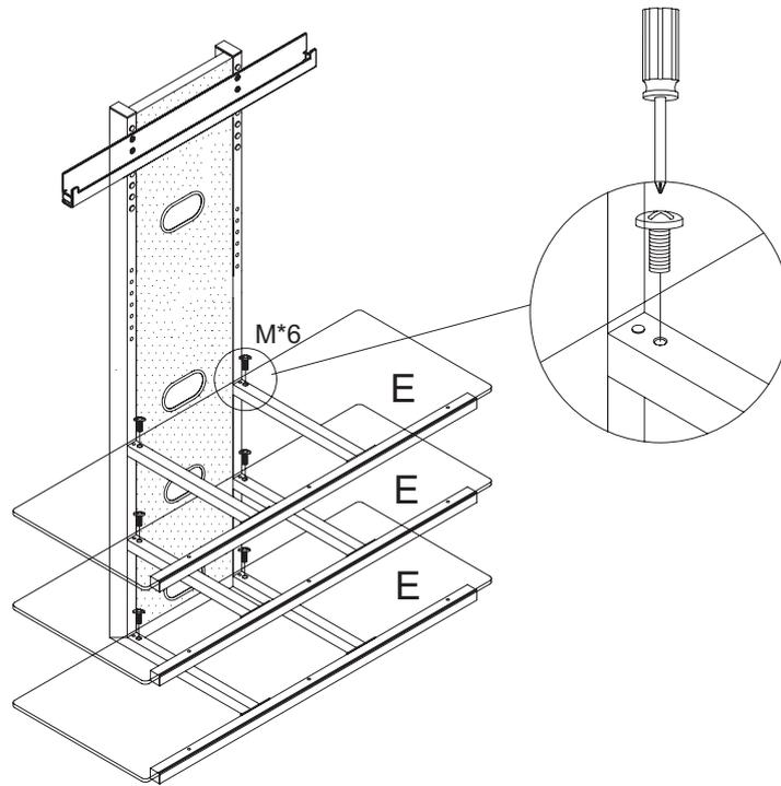
5-Fasten the glass (E) on the beams with screws (M). Do not over tighten screws.
