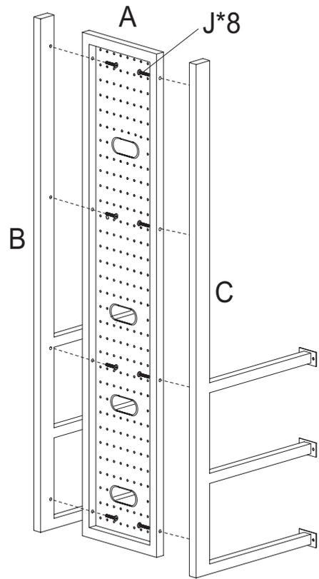
1-Attach frames (B) & (C) to the back panel (A) with screws (J).
