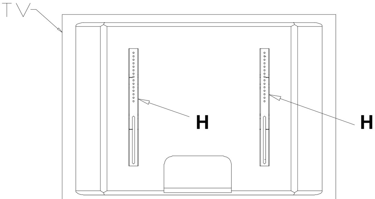
6-Fasten two TV mounting brackets(H) on the back panel of the TV. Detail assembly instructions refer to next pages.
