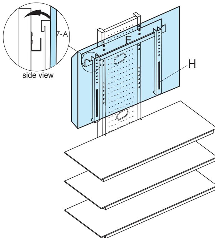
8-After mounting the brackets (H) to TV, hang TV onto holder (F), see (7-A).
