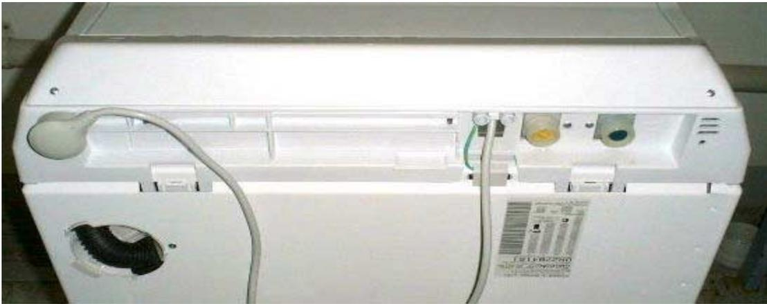
3. Remove the 2 screws from the rear of the top console, disconnect the earth lead. The console can now be raised for access to the Motor Controller Module, Display Module and associated wiring.
