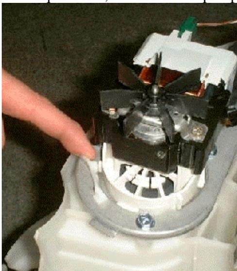
To remove the pump, turn it towards the front of Smartdrive until the locking tab prevents further turning, then release the locking tab by pulling it away from the pump. Continue to turn, the pump will disengage. When refitting the pump, making sure that the bayonet fixture is located correctly. Twist the pump away from the front of Smartdrive until the locking tab clicks into place.
