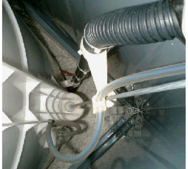
**Drain Hose.** Unclip the drain hose fixture from the lip of the outer bowl and screw into position on the cabinet. Ensure the drain hose grommet is correctly fitted, (photo).
