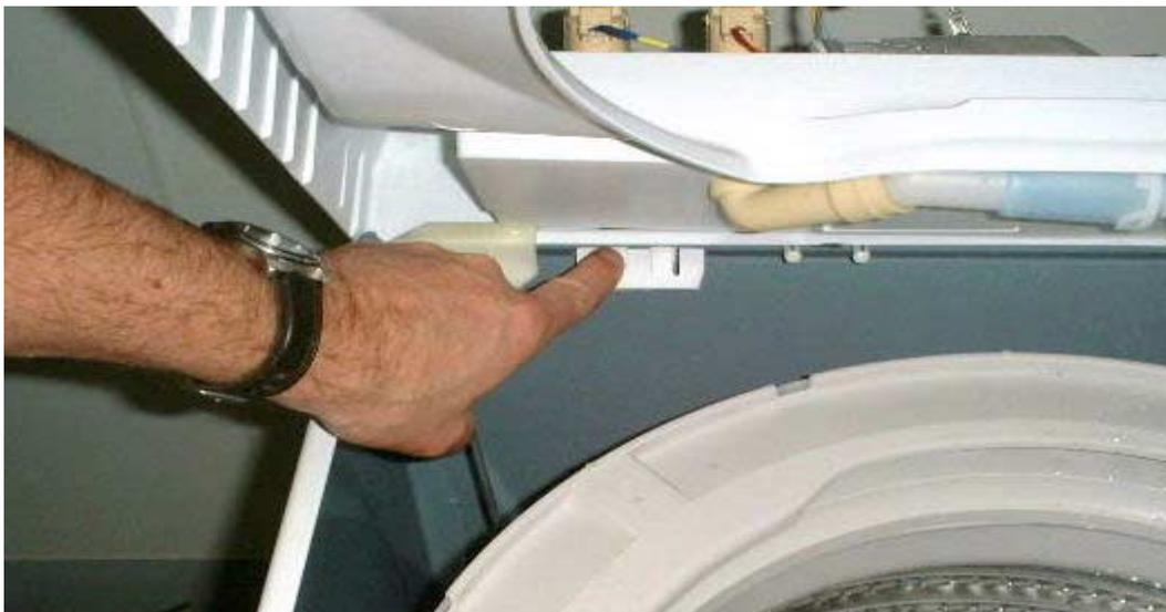
**NB:** The top deck cannot be hinged back without first releasing the rear clips from the cabinet and lifting at the same time.
