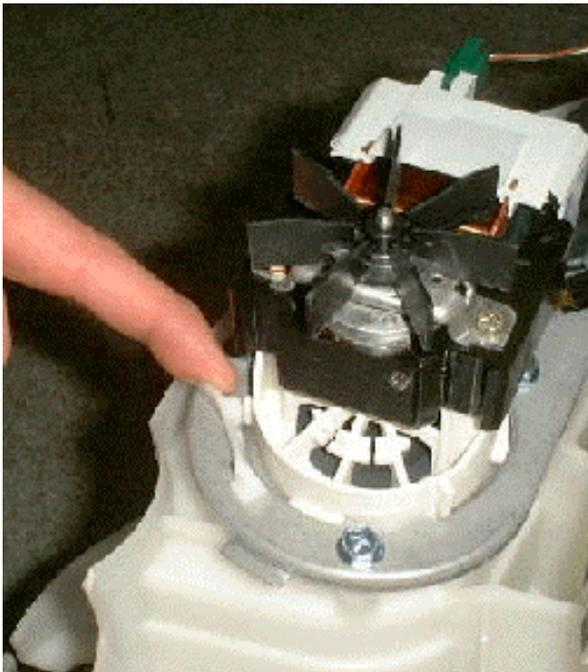
15. To remove the pump, release the locking tab. Turn the pump anti-clockwise, lift it clear and remove the electrical connections.
