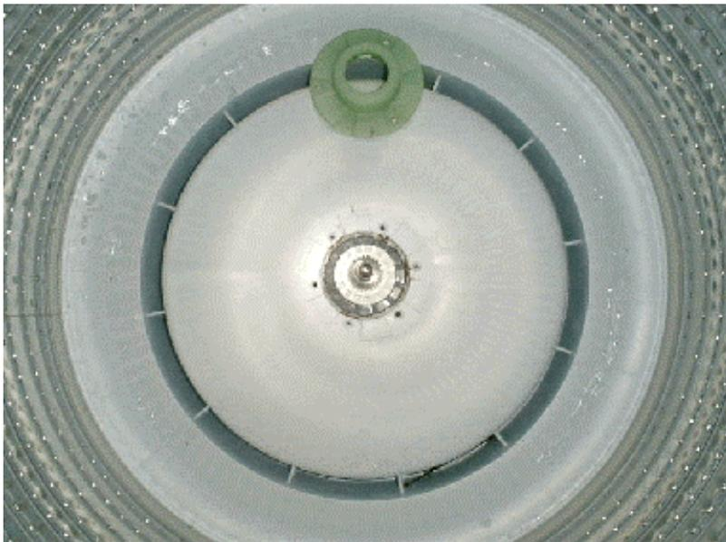
If not already removed, the clutch can be disassembled at this stage by removing the three screws from the driven spline.
