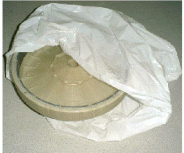
**NB:** When placing the stator on a work bench, ensure the RPS connectors are facing upwards or damage can result. **Do not place the stator inside the rotor.**
