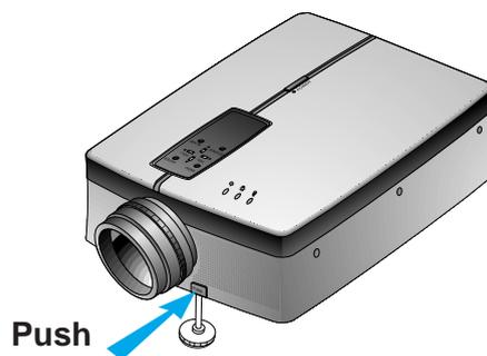
1. Press the foot adjuster button while you support the other side of the projector. This unlocks the foot and can make it move freely. Take care not to drop the projector.
