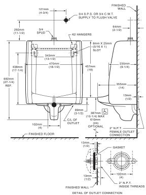
**NOTES:** FLUSH VALVE NOT INCLUDED AND MUST BE ORDERED SEPARATELY. PROVIDE SUITABLE REINFORCEMENT FOR ALL WALL SUPPORTS.
