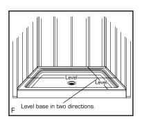
rough floor along the entire length of the shower base. Insure that the base is level in two directions (see Fig. F). Snap strainer back into place and check for proper drainage.
