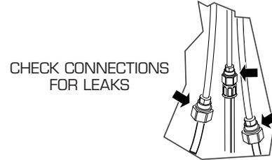
CHECK CONNECTIONS FOR LEAKS
