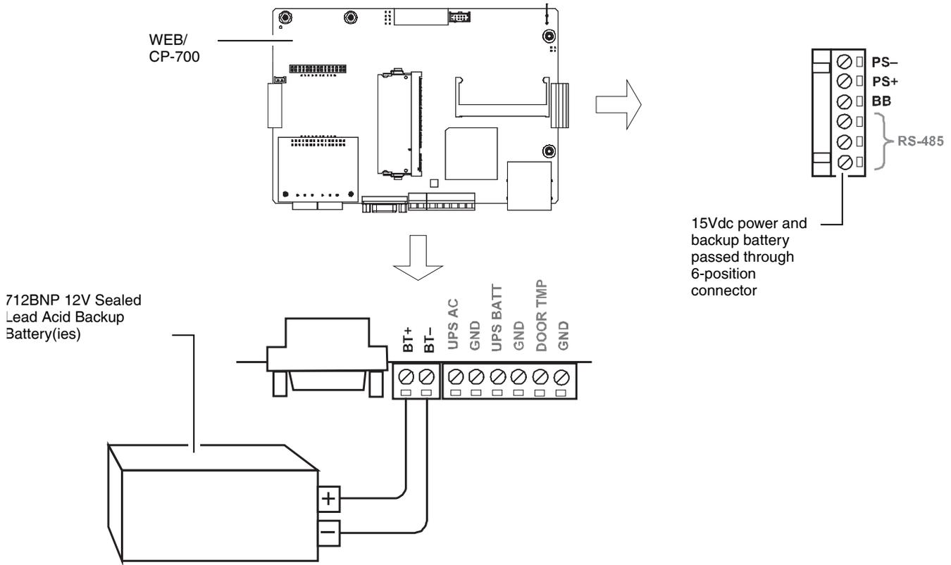
Fig. 10. Sealed lead-acid backup battery connection on WEB/CP-700.
