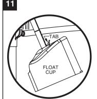
Turn on water supply. Let the toilet cycle once. Adjust the water to desired level by depressing TAB on FLOAT CUP and moving FLOAT CUP up or down.
