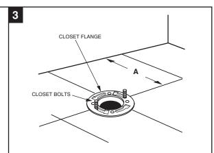
**INSTALL CLOSET BOLTS** Install closet bolts in flange channel and slide into place parallel to wall.
