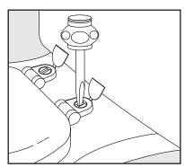
Use a screwdriver to tighten bolt.
