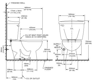
THIS COMBINATION IS DESIGNED TO ROUGH-IN AT A MINIMUM DIMENSION OF 305MM (12") FROM FINISHED WALL TO C/L OF OUTLET.
