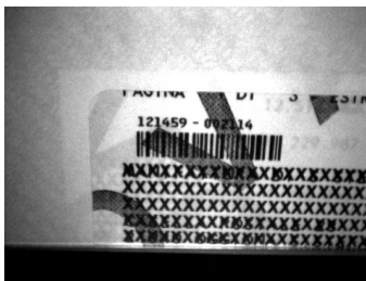
Figure 3 - Overprinted Barcode Readable by Matrix-1000™ also Through the Envelope Window Film
