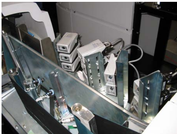
Figure 5 - Ten readers connected to a Datalogic MX4000 through a multidrop network.
