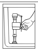
Turn on water supply. Adjust water to desired level by squeezing water level adjustment clip and moving FLOAT CUP up or down along stainless steel link.
