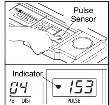
indicator in the pulse display flashes **steadily**. Hold your thumb at this level. After a few seconds, three dashes will appear in the display and your pulse will be shown. Hold your thumb on the sensor for another 15 seconds for the most accurate reading. If the displayed pulse appears to be too high or too low, or if your pulse is not displayed, lift your thumb off the sensor and allow the display to reset. Press down again on the sensor as described above.
