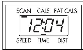
When the power is turned on, the Scan mode will be selected. One mode indicator will appear by the word SCAN, and another mode indicator will show which mode is currently displayed.
