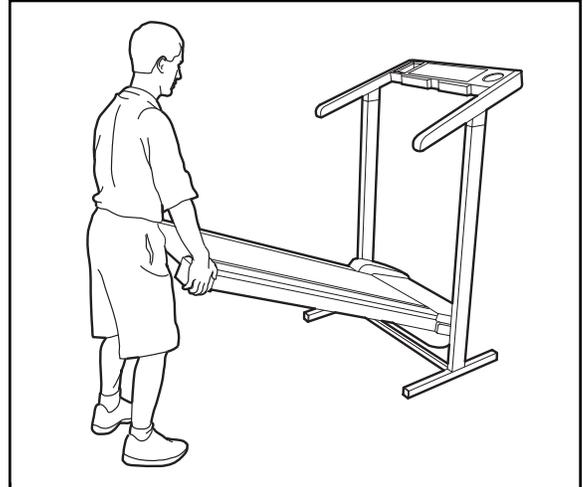
2. Move your right hand to the position shown at the right, and hold the treadmill firmly. Raise the treadmill until the storage latch locks over the frame guide. **Make sure that the storage latch closes fully over the frame guide.**
