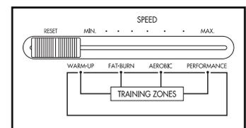
Next, slowly move the speed control until the walking belt begins to move at slow speed. Carefully step onto the walking belt and begin exercising. Change the speed of the walking belt as desired by moving the speed control.
