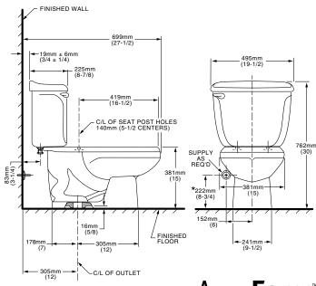
THIS COMBINATION IS DESIGNED TO ROUGH-IN AT A MINIMUM DIMENSION OF 305MM (12") FROM FINISHED WALL TO C/L OF OUTLET.
