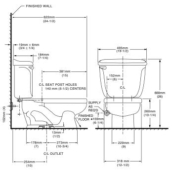
NOTES: THIS COMBINATION IS DESIGNED TO ROUGH-IN AT A MINIMUM DIMENSION OF 254mm (10) FROM FINISHED WALL TO C/L OF OUTLET \* DIMENSION SHOWN FOR LOCATION OF SUPPLY IS SUGGESTED. SUPPLY NOT INCLUDED AND MUST BE ORDERED SEPARATELY.
