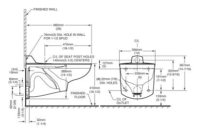
● Toilet designed to meet ADA accessibility standards when top of seat height set at 432 to 483mm (17" to 19") from finished floor.
