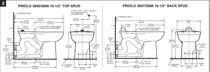
**DIMENSIONS (Nominal)** NOTE: Distance from floor to closet flange centerline (rough-in) must be 4" (102 mm) with flange surface flush to 1/16" (1.6mm) max. beyond finished wall.
