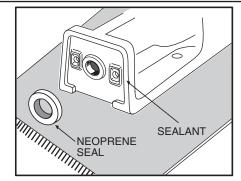
INSTALL NEOPRENE OR GRAPHITE FELT SEAL\*
