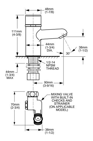
NOTE: Dimensions are shown for product installed less escutcheon.
