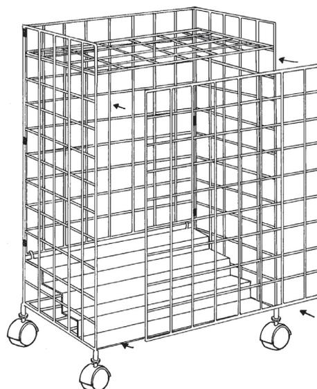
4. Attach front grid (D) to side grids (A). Using small clips, attach grid (C) to grids (A).
