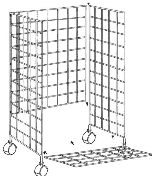
2. Using large plastic clips, attach one large grid (A) to the back grid (B), then attach the other large grid (A) to the other side of grid (B). Attach center grid (C) to bottom.
