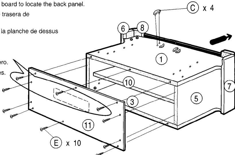
For ease of installation, screw in the top 3 holes first, before attempting to screw in the side and bottom screws.
