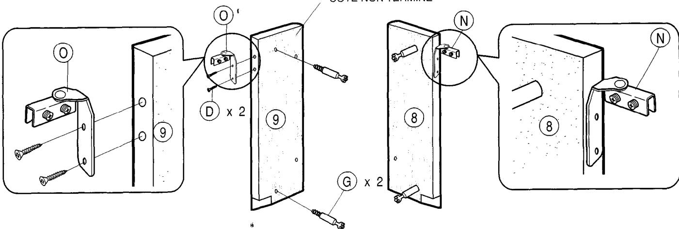
Insert 2 connecting bolts to both the right and left front panels. Attach hinges accordingly by screwing in screw (D).
