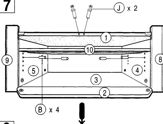
Screw in 2 magnets (J) into embedded magnet sleeves in top board.
