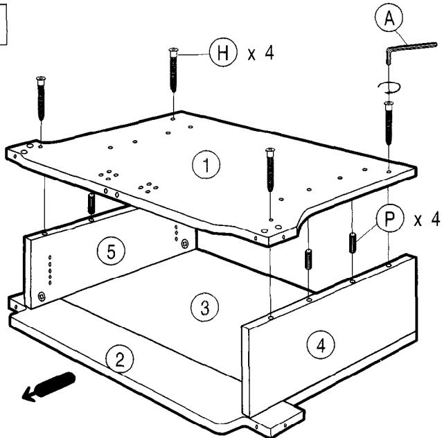
Insert 2 dowels into each side board. Attach top board by using 4 hex. screws.
