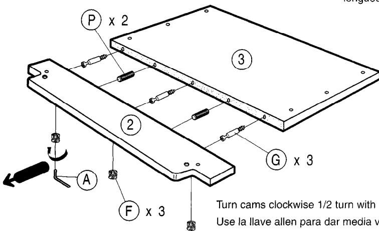
Insert 2 dowels to about 1/2 their length. Use hammer lightly if necessary (rubber mallet suggested).
