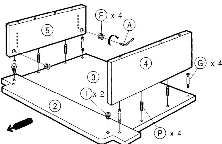
Turn cams clockwise 1/2 turn with allen wrench to lock panels together.
