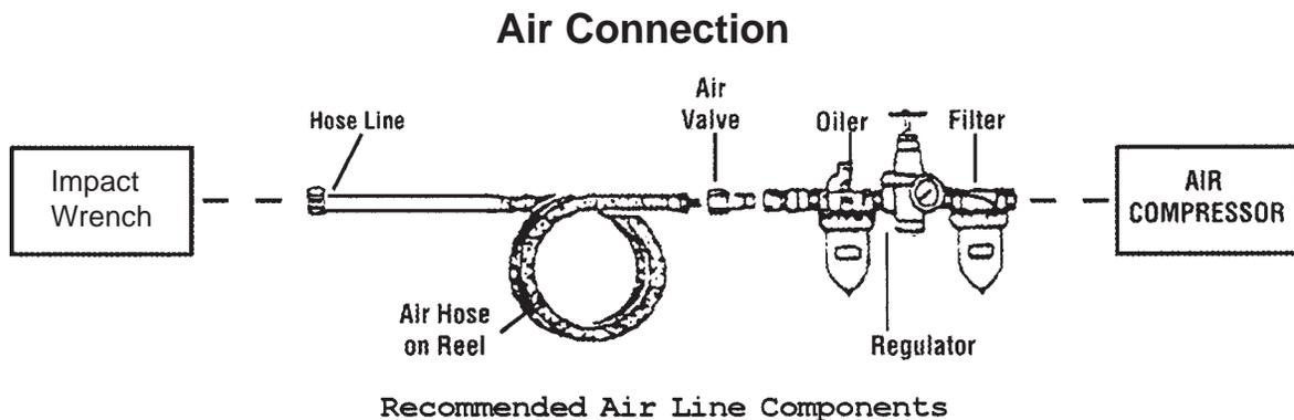
For best service you should incorporate an oiler, regulator, and inline filter, as shown in the diagram above. Hoses, couplers, oilers, regulators, and filters are all available at Harbor Freight Tools. For optimal performance, use an air compressor of 15 Horsepower or more and limit the total air line length to 30' or less.
