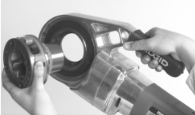
Figure 3 – Installing No. 11-R Die Heads
