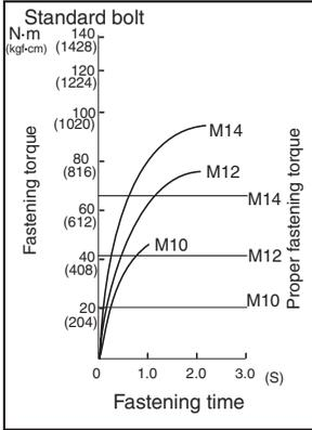
The proper fastening torque may differ depending upon the kind or size of the bolt, the material of the workpiece to be fastened, etc. The relation between fastening torque and fastening time is shown in the figures.
