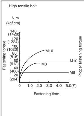
The fastening torque is affected by a wide variety of factors including the following. After fastening, always check the torque with a torque wrench.
