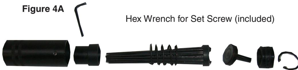
1. Insert the Needles (5A) through the holes in the Needle Holder (4A). There are nineteen Needles. Make sure all holes are filled before putting the Needle Holder (4A) through the Spring (3A), the Retainer Clip (2A) and into the Barrel Assembly (1A). Slide one Retainer Ring (8A) around the Needles (5A) and fasten it at the front end of the Barrel Assembly (1A). See **Figures 4 & 4A**
