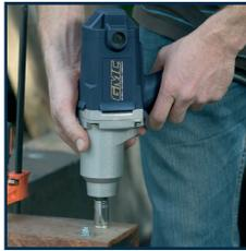
2. Depress the switch and fasten for the fastening time.
