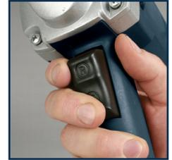
**CAUTION.** Always maintain a tight control of the tool when switching on and off. Remember the motor will continue to run for a short time after switching off.
