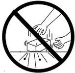
Handle the receiver gently and carefully. Dropping it can damage its circuit boards and can cause the receiver to work improperly.
