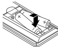
Remove the battery cover on the rear of the remote control, and insert two R03 (size AAA) batteries with ⊕ and ⊖ aligned correctly.
