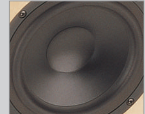
SHIELDED LONG THROW DRIVER WITH COATED MULTI-FIBRE PAPER PULP CONE.
