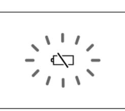
will be displayed on the LCD screen. Replace with a fully charged battery.
