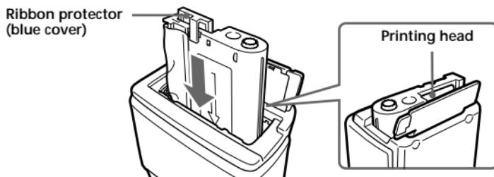
The ribbon protector is located between the ribbon and the cartridge case. This protector prevents the ribbon from being tangled when inserting the print cartridge into the cartridge compartment.
