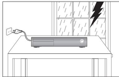
During thunderstorms, disconnect the AC main plug from the wall outlet. Voltage peaks due to lightning could damage the unit.
