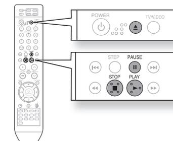
**To stop playback, press the STOP (⏏) button during playback.**
