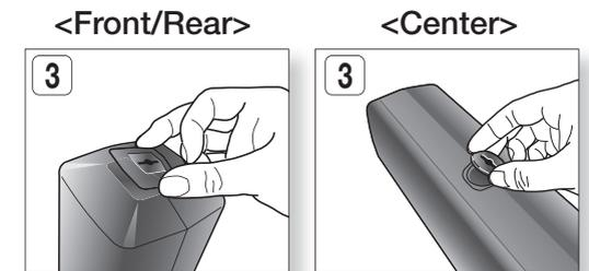
4. Use a coin turn the hole cover clock wise to fix it. (Turning it counter-clock wise will loosen from the hole.)
