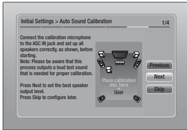
13. The Auto Sound Calibration screen appears. Plug the ASC microphone into the ASC IN jack on the product.
