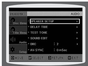
**4** Press Cursor **▲, ▼, ◀, ▶** buttons to move to the desired speaker and then press **ENTER** button.
