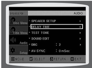
**4** Press Cursor  $\blacktriangle$ ,  $\blacktriangledown$ ,  $\blacktriangleleft$ ,  $\blacktriangleright$  buttons to move to the desired speaker and then press ENTER button.
