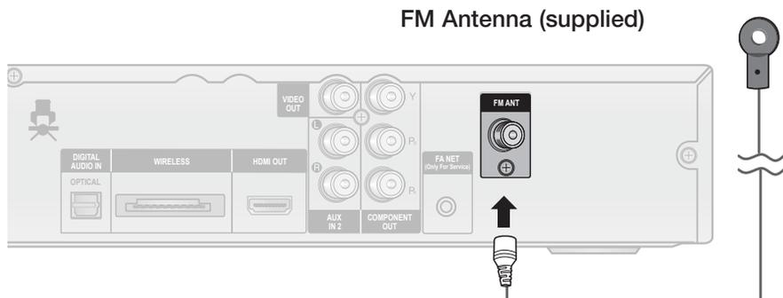
1. Connect the FM antenna supplied to the FM Antenna jack.
