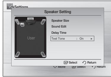
Use the Test Tone feature to check the speaker connections.
