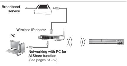
You can connect to network with a Wireless IP sharer. A wireless AP/IP router is required to make a wireless network connection. Set the network options. (See page 39)
